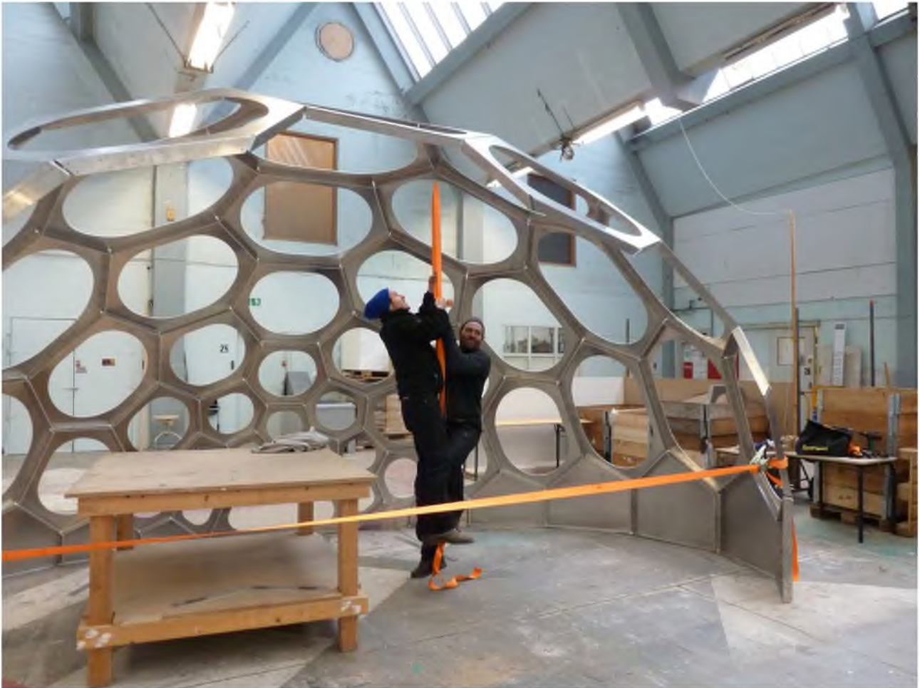
Figure 25: Testing of concentrated load load on vertex.
