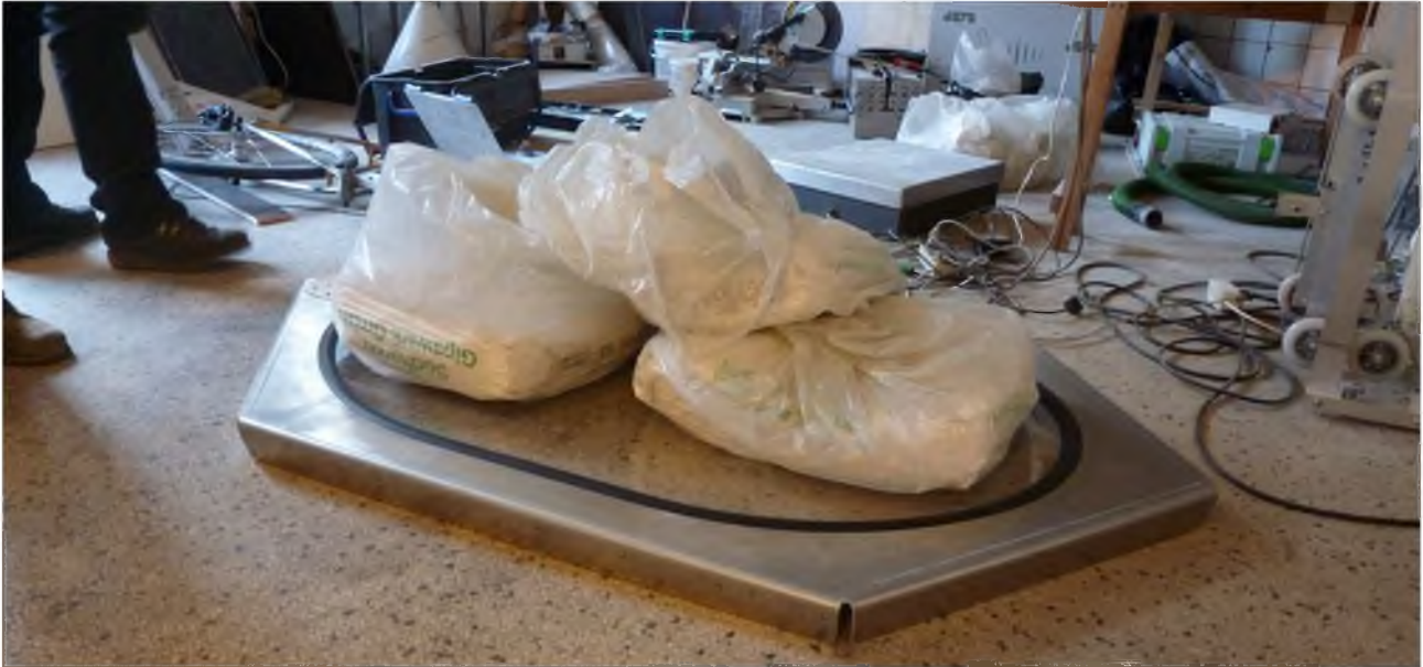
Figure 23: Physical load test of the largest plate.
