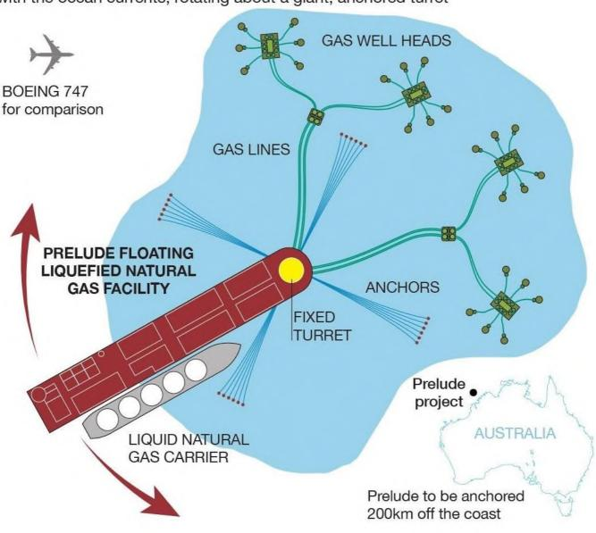
"Aligning with the prevailing wind, waves or current, while the turret moorings remain fixed to the sea floor, ensures Prelude can remain safely at its location through the most powerful cyclones," says van Loon.
