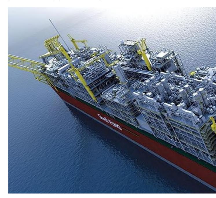
By the numbers, the largest ocean-going vessel ever built is a mind-boggling beast. Stretching half a kilometre from bow to stern, and with a superstructure that will eventually soar 30 storeys above the waterline, the 600,000-tonne Shell Prelude displaces as much water as six aircraft carriers. But it is by its
